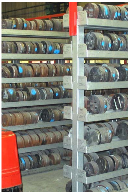
Kaye Aluminium carries a large stock of the customer specific dies essential to the extrusion process.
