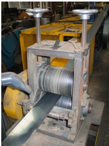
Strip being continuously hardened and tempered.
