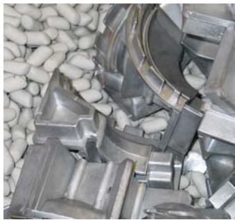
Die-cast components are de-burred using specialist treatments
